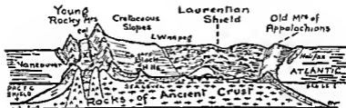
FIGURE 10—Profile section of Southern Canada (much generalized) A series of weak sediments originally deposited in a wide Cretaceous trough was buckled up (early in Tertiary times) between the Pacific and Laurentian Shields and formed the Rockies These have been greatly eroded and the old core rocks exposed In the east the old Appalachians were lifted en masse without folding (K = Kamloops)
